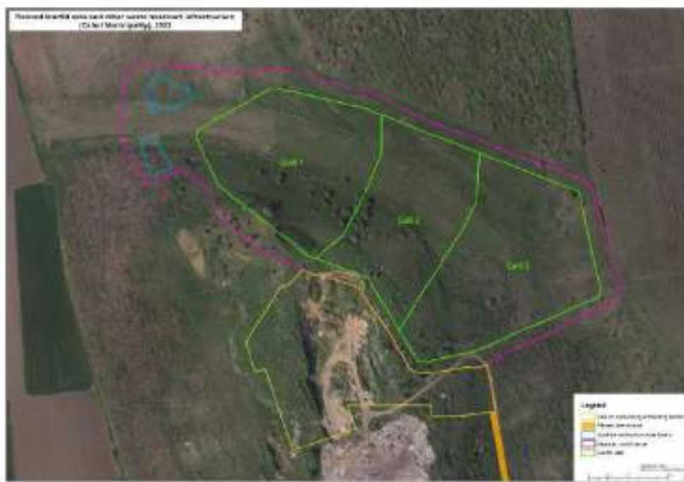
Figure 3.9 A detail of the Cahul site with the indicated layout of proposed regional sanitary landfill for WMZ-1
