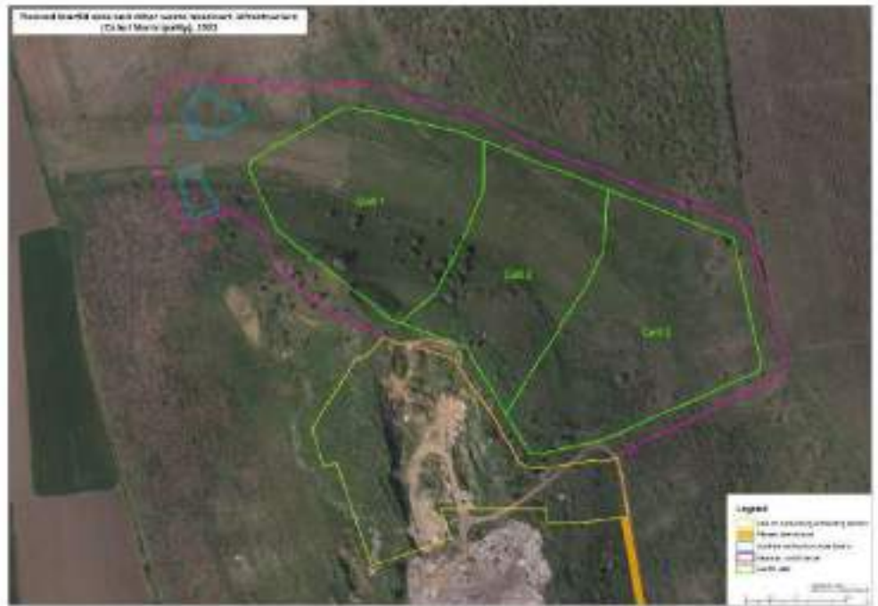
Figure 5.7 A detail of the Cahul site with the indicated layout of proposed regional sanitary landfill for WMZ-1
