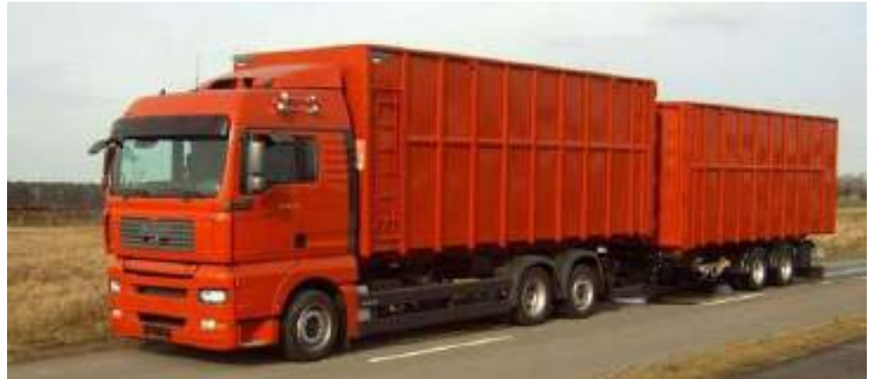
Figure 2.5 Example of truck-and-trailer vehicle for long-distance transportation of waste from TS to WMC
